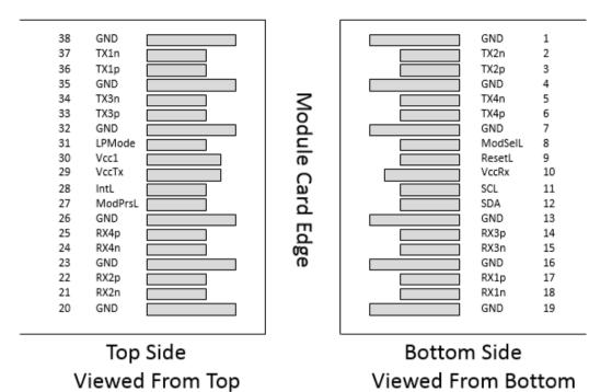
Figure 2. MSA compliant Connector
