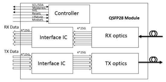
Figure 1. Transceiver Block Diagram
