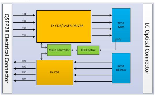
Figure 1. Transceiver Block Diagram
