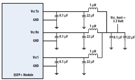
Figure 3. Recommended Power Supply Filter
