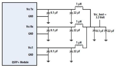
Figure 3. Recommended Power Supply Filter
