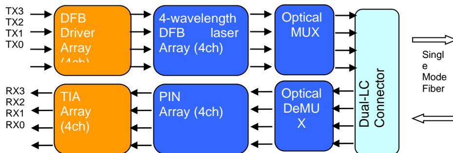
**Figure 1: 40Gb/s QSFP IR4 Transceiver Block Diagram**
